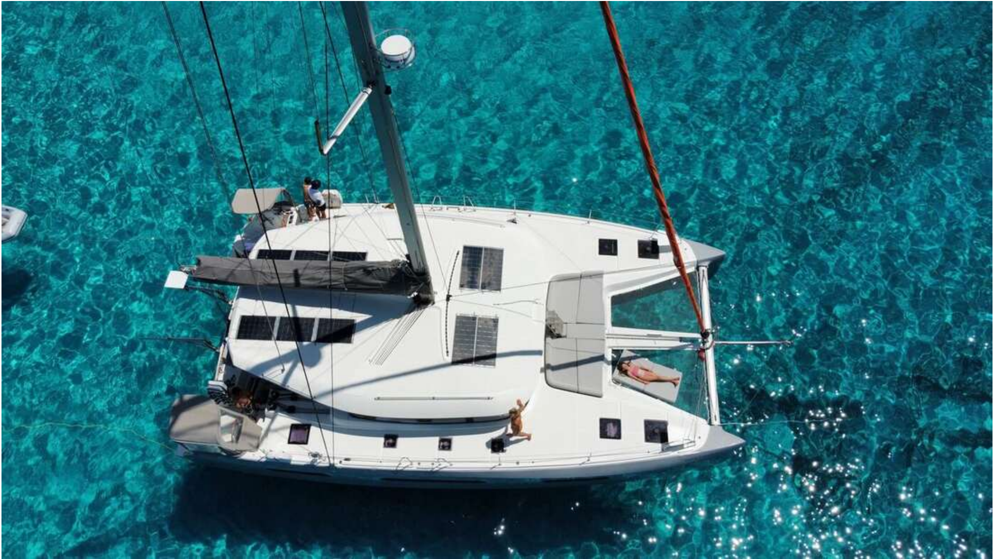
Deck plan from above: solar panels, boom bag, trampolines and cockpit
