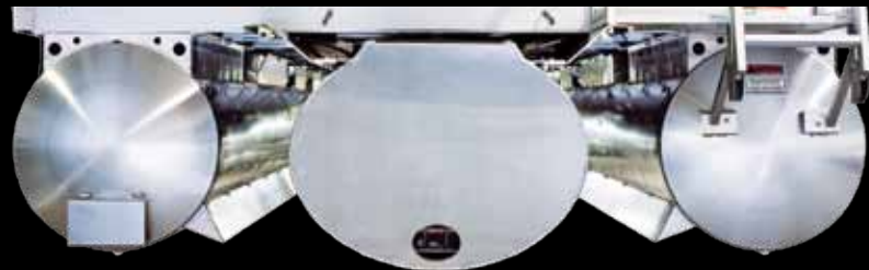
A 32" center elliptical tube with lifting strakes and twin 25" tubes with performance foils provide high performance banking in tight turns.
