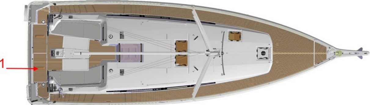
The liferaft (not supplied) must be stored in the space provided for it (Ref 1).
