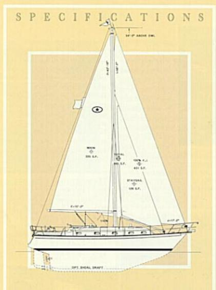
LOA 39'7" (12.06 m) Displacement (approx.): LWL 32'0" (9.75 m) 21,000 lbs. (9,526 kg) Beam 13'2" (4.01 m) Ballast 9,000 lbs. (4,082 kg) Draft 4'7" (1.40 m) Sail Area 885 ft1 (82.22 m1) (Shoal Option) 3'11" (1.18 m) Sail Area/Displ. 18.6 Mast Above DWL 54'3" (16.54 m) Displ/Length 286 Fuel 85 gal. U.S. (3221) Ballast/Displ. 43% Water 170 gal. U.S. (6441) Auxiliary Power: Headroom 6'5" (1.96 m) 56 hp FWC Diesel (41 kw) Cabins/Berths 3/7
